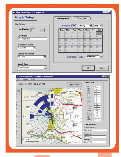
'Live' sensor readings can be displayed as digital meter type graphics, and historical data is easily produced using the calendar start / end date and time window as shown above.
